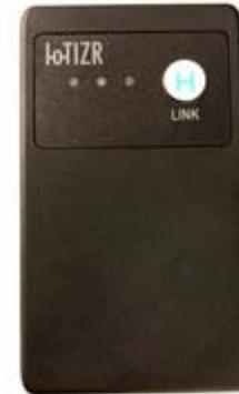
IoTIZR: Our original device to connect water flow meter and transfer via Wifi
